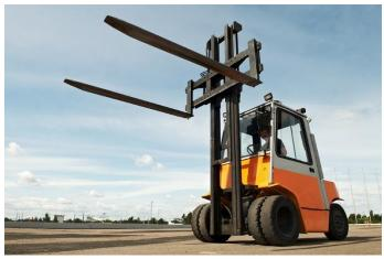
Hydrogen H<sub>2</sub> Materials handling - Fuel cell industrial trucks, like forklifts or towing trucks, are especially suitable for indoor operation, because they produce no local pollutant emissions and only low noise emissions. Fuel cell vehicles have advantages over battery operated industrial trucks in terms of refuelling. Instead of having to replace the battery, the trucks can be refuelled within two to three minutes. They take up less space and are cheaper to maintain and repair.
