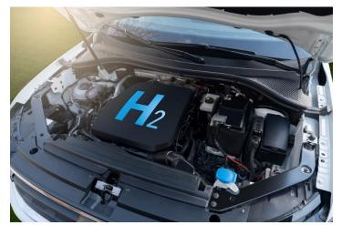
Light Vehicles - Along with battery electric vehicles, hydrogen powered fuel cell passenger cars are the only zero emission alternative drive option for motorized private transport. The fuel cell stacks in the latest fuel cell models have an output of 100 kW or more.
